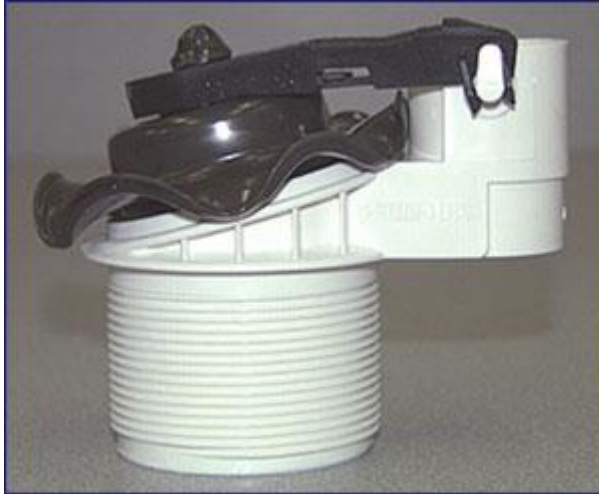
Figure 1: Deformed flapper valves are often the result of toilet tank cleaning products. (Photo courtesy of John Koeller & Company)
